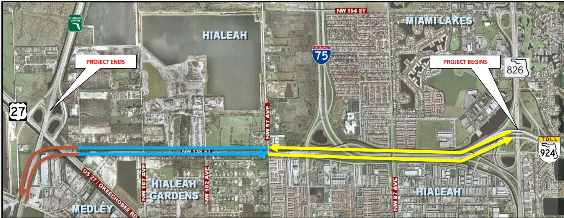
Two-lane ramps to and from the south only, will connect Florida's Turnpike with the NW 138<sup>th</sup> Street corridor providing a direct connection west of NW 107<sup>th</sup> Avenue.
